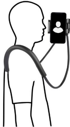
Figure 4. SuAvE Design utilizing a neck harness as the accessory for holding the personal electronic device.
