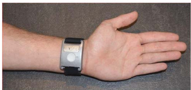
Figure 1. Photograph of a Q-sensor used to access the skin conductance levels of staff members during a day, evening, and night shift
